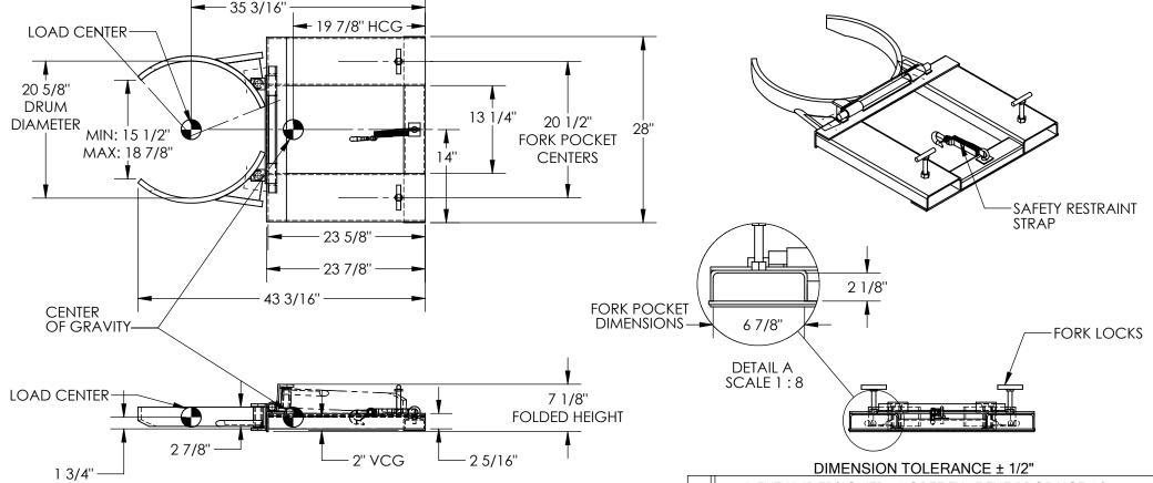
STANDARD FEATURES MODEL NUMBER IS DGS-55-D **OVERALL WIDTH IS 28" USABLE WIDTH MIN: 15 1/2"** MAX: 18 7/8" **OVERALL LENGTH IS 43 3/16" USABLE LENGTH IS 23 5/8"**
